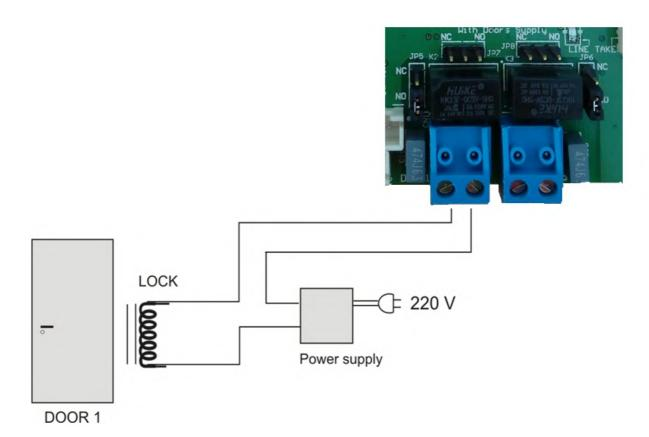
Other configuration is possible as you can see in the following picture. In this case, the same power supply is used, for both, electronic board and door lock:
